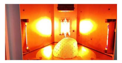
Image: Orion's Additive Manufacturing System for PEEK
